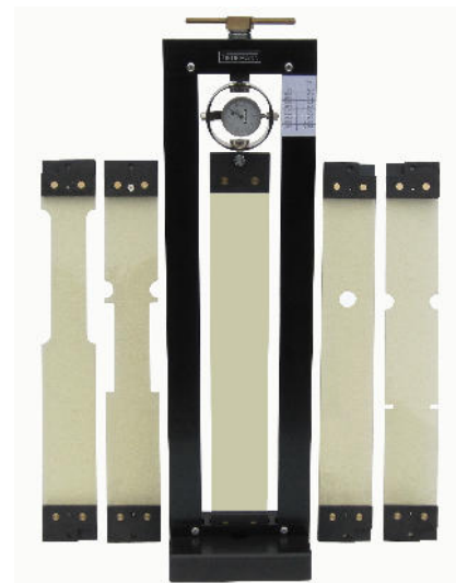
Tension force frame with dynamometer and five models
