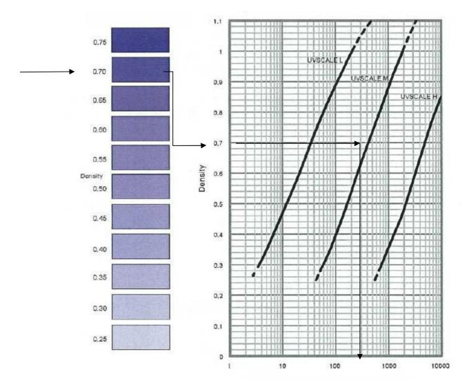
Compare the obtained measurement film with the colour samples on the left. Then the respective calibration curve/film type can be found and its ultraviolet light dose can be read on the abscissa.
