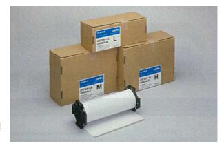
The UV-light measuring film can be equally prepared as the heat flux film Thermoscale or pressure measuring film Prescale. Cut with scissors it is placed on the body to be tested. Within the film are microcapsules and color developer which react to exposure to and stain the slide. The intensity of the color is proportional to the amount of UV light dosage.
