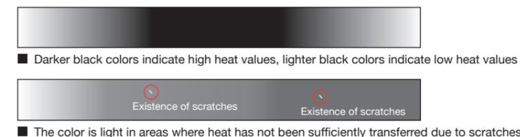
The color is light in areas where heat has not been sufficiently transferred due to scratches, etc.
