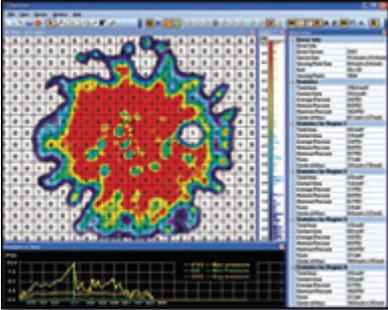
The architectural philosophy of Tactilus<sup>®</sup> is modular allowing for portability, easy expansion, and simultaneous data collection of up to 4 discrete sensor pads. Tactilus<sup>®</sup> employs sophisticated mathematical algorithms that intelligently separate signal from noise, and advanced electronic shielding techniques to maximize the sensor’s resistance to noise, temperature and humidity.
