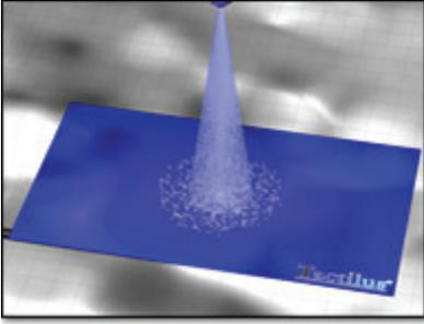
Our Tactilus<sup>®</sup> spray sensor reveals contact impact pressure distribution and magnitude across the entire surface area of your spray surface. Now for the first time you can verify FEA and CFD analyses with data gathered directly from your contact surface.
