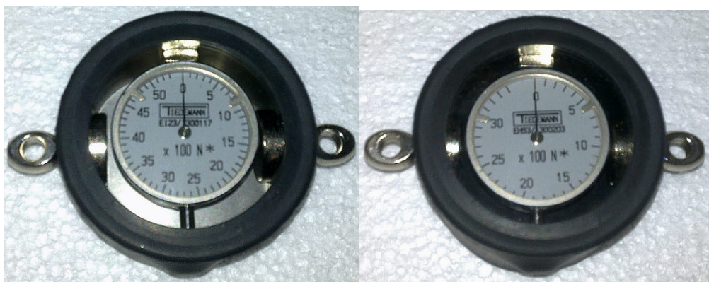
Dynamometer for Y-Cable Tensioning Device with up to 5 kN and 3.5 kN
