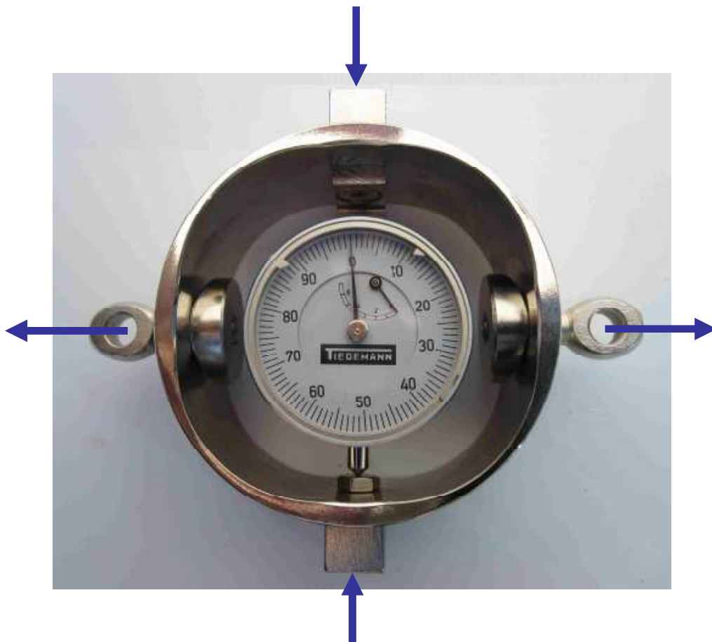
Universal Analogue Dynamometer with standard scale, max 2 kN
