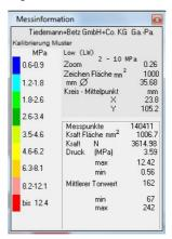
The footprint images are scanned to measure the intensity of colour change. The program then returns to the calibration curve defined for each type of film for smooth surfaces at room temperature and specific humidity. If the measuring conditions deviate from this or if the surface is structured, calibration curves can be prepared in advance.
