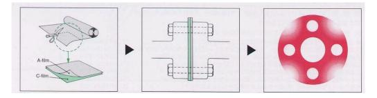
With increasing load, no reaction will appear in any given film type and then if the load increases and the first micro-capsules burst, the
