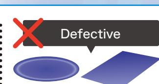
Defective if the coloring is uneven. Coloring that is lighter than previously also indicates that the light source may have deteriorated.
