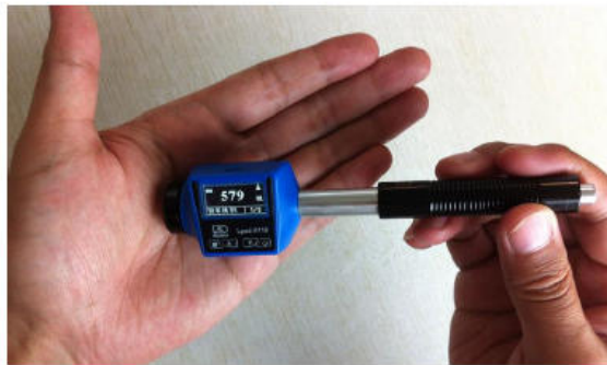
Leeb hardness measurement principle
