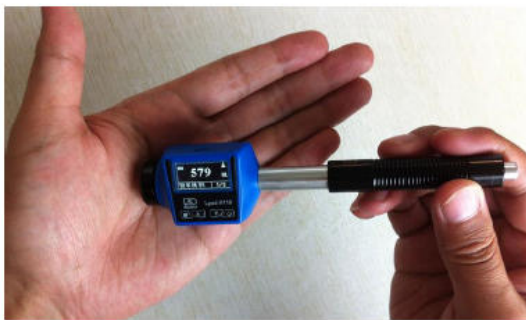
Leeb hardness measurement principle
