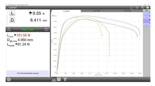
With the L2/S1 software, pre-configured tests are simply provided with the desired parameters or you can create your own test sequences with the configurator.
