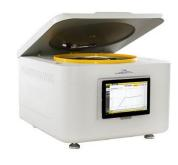
software which supports automatic controlling of temperature, humidity and flow rate precisely and guarantees the testing sensitivity and repeatability of the test results. C360H is applicable to determination of water vapor permeability of plastic films, sheeting, paper, packages and other packaging materials in food, pharmaceutical, medical apparatus, building materials and consumer goods, etc.
