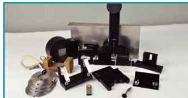
Different kinds of fixtures to measure different kinds of samples.
